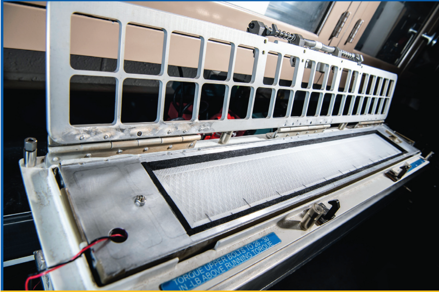
A Multi-Stage Filtration System for the International Space Station that collects dust and other particulates was invented by Glenn's Juan Agui. Photo Credits: NASA/Jordan Salkin
